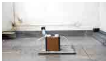
Overcharge non-thermal runaway electrical performance test
