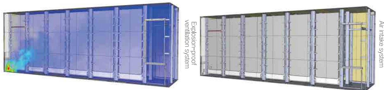
Figure 19 Combustible Gas Concentration in the Cabinet Minutes after Mechanical Exhaust System Activation
