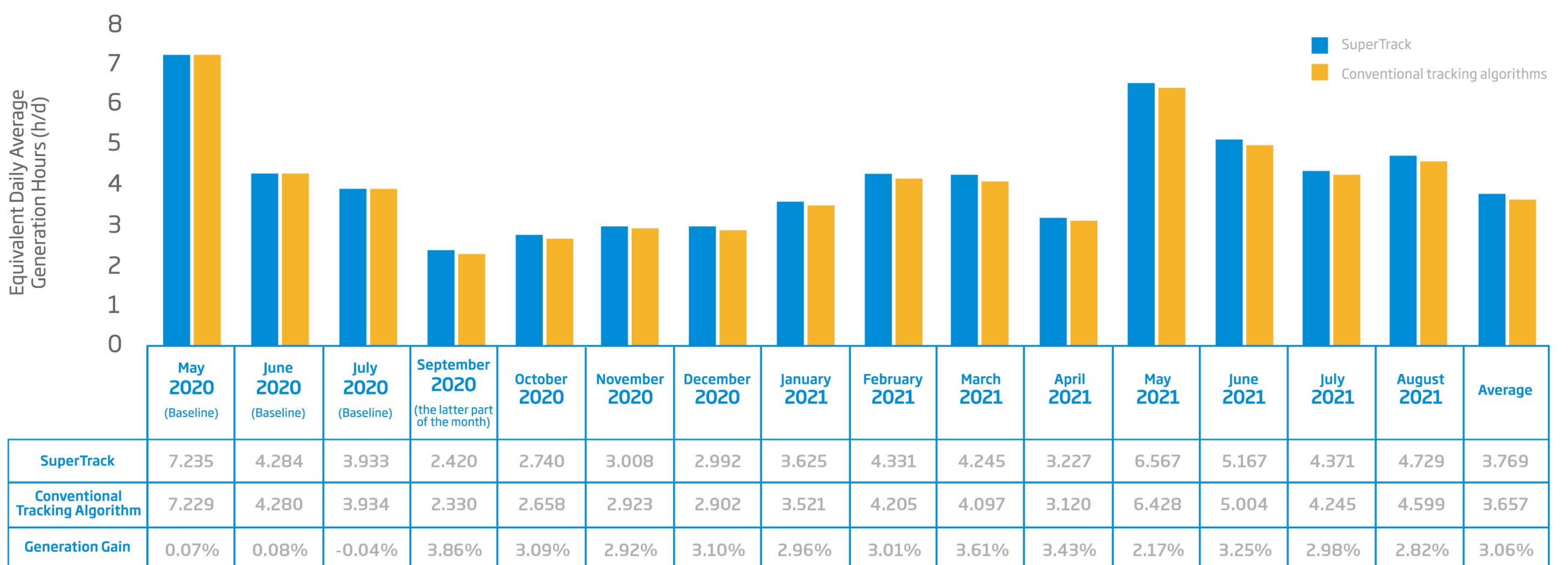
Comparison of the equivalent power generation hours and power generation gains for different months in the Tongchuan project
