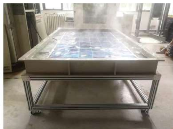
PID test device (60°C、75°C、85°C、3.5% saline soak PID)
